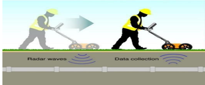
Picture No. 2.2.2: Schematic representation of GPR survey
